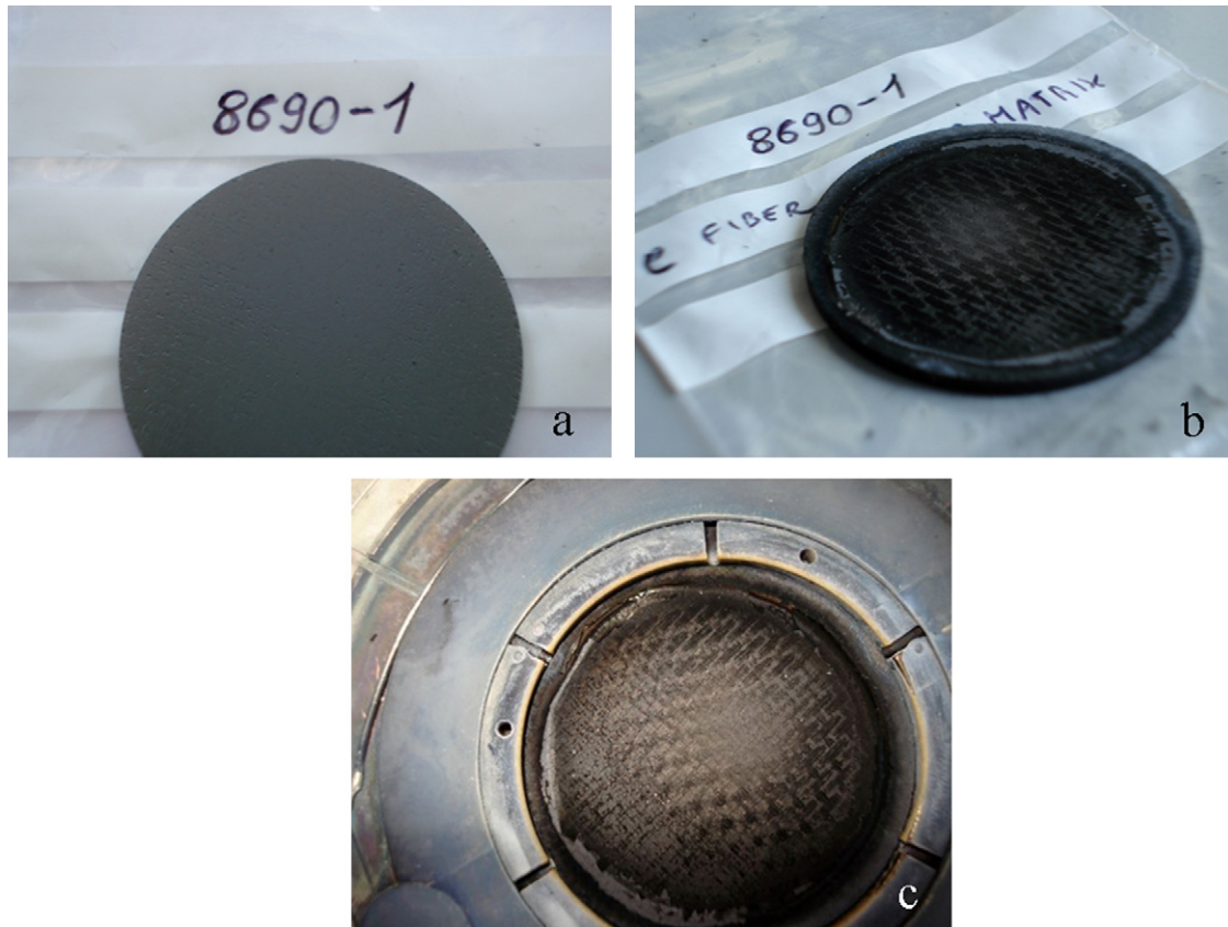
Fig. 3. Pictures of the emitting surface of the sample CVD SiC-coated C/SiC (a) before and (b) and (c) after the emissivity experiment carried out increasing the temperature from 600 °C up to about 1600 °C at air pressure of 200 and 4 Pa, respectively.
